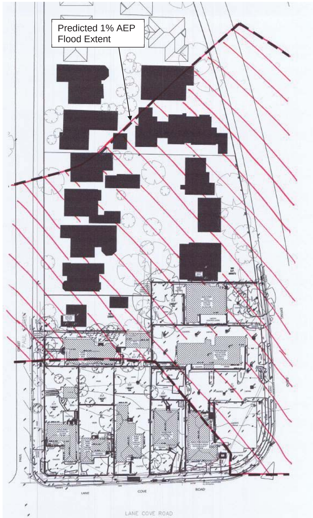
Figure 2 – Existing Flood Storage Area
